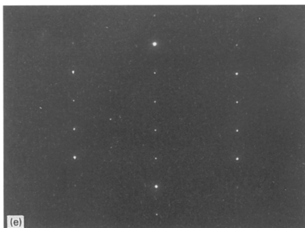
Figure 7 In situ observation of high-temperature transformation of large quasicrystals. The SAD pattern (e) corresponds to the [010] zone axis of the \text{Al}_{13}\text{Fe}_4 phase (see text for details).
